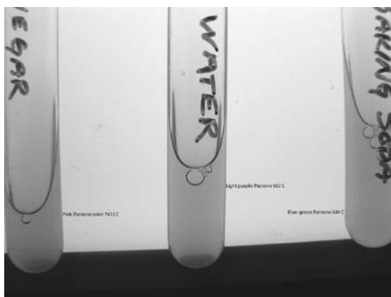
FIGURE 3.17 The Three pH Standards After the Addition of Red Cabbage Juice
