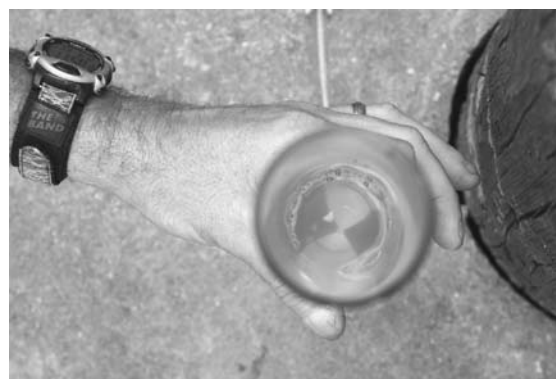
FIGURE 3.15 Turbidity Tube Showing Visible Secchi Disk at Bottom of Tube
