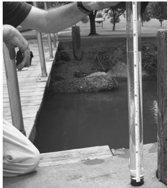
FIGURE 3.15 Turbidity Tube Showing Visible Secchi Disk at Bottom of Tube
