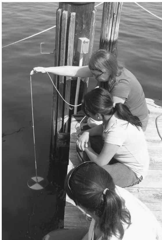
FIGURE 3.13 Using a Secchi Disk to Measure Transparency
