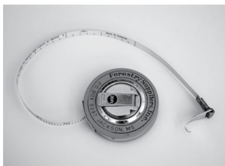
Figure 4.6. Instruments for measuring tree DBH. Top—tree calipers; bottom—diameter tape (D-tape).
