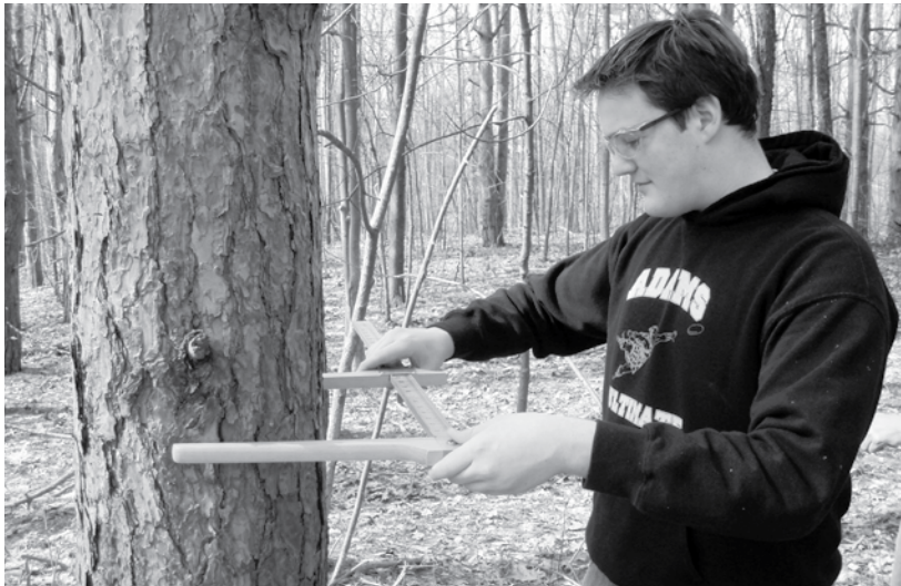
Figure 4.7. Using tree calipers to determine tree DBH.
