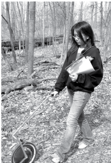
Figure 4.1. Using a distance measuring wheel to determine the perimeter dimensions of a study plot.
