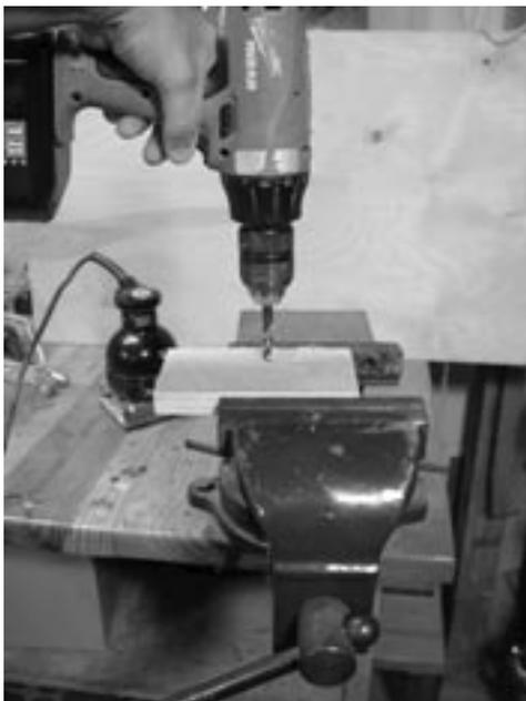
Using a vise is the safest and most secure method for holding pieces of wood during construction.
