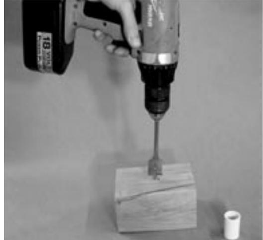
2. The coupler should fit snugly into the hole drilled in the block. The end cap will occasionally hit this coupler during the operation. It will become dislodged if it is not securely attached within the block. If the connector is too tight to push in by hand, tap it with a wooden block to push it into place.
