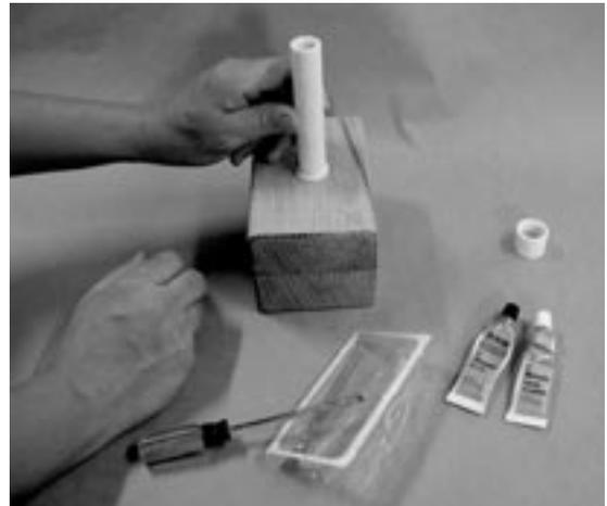
9. After the glue has dried, the block should slide on the tube with some effort. If it is too hard to move the block, it can be made easier by sanding the inside of the PVC coupler. Do not make it too easy, or the demonstration will not work. Varnish the block to seal the wood and give it a nicer appearance.
