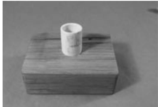
3. If the drilled hole is not quite large enough, sand the inside of the drilled hole until it is the right size. To do so, wrap a piece of sandpaper around a wooden dowel and use a rubber band to hold it in place. This sanding stick can be used with the drill to sand the inside of the block. Use the drill on high speed to get a smooth, rounded hole.
