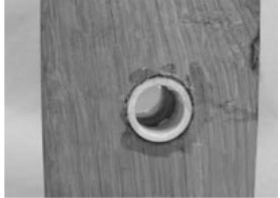
8. If 2 coupler pieces are needed, insert a piece of PVC piping through both couplers while gluing the second piece in place. This will help ensure they are aligned properly. Glue the other half of the coupler into the opposite side of the block. Once again make sure that the edge of the coupler is flush with the wooden surface.
