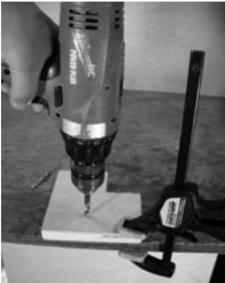
Using a clamp or clamps is one alternative to holding parts by hand. Several types of clamps are available and can be found in most hardware stores. The wood is shown clamped down to a workstation. This is more secure and safe than holding it in your hand and will yield greater precision in cuts and drilled holes.
