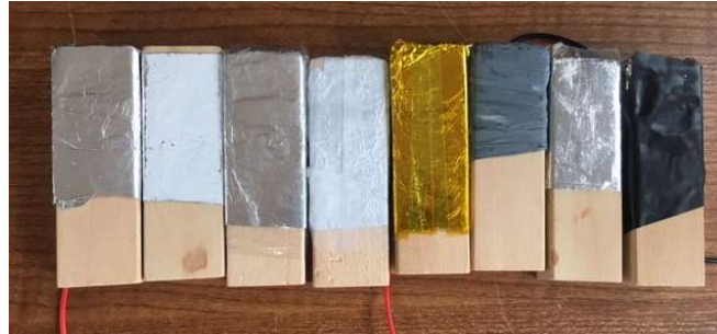
Different electrodes made using Jenga blocks
