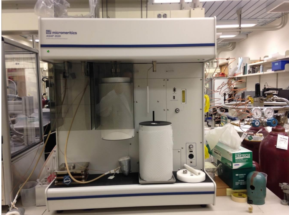
Figure 7 Micromeritics ASAP 2020 Surface Area Analyzer at Battelle.
