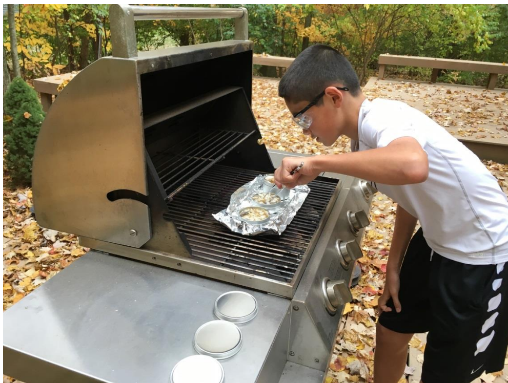
Figure 10 Heat treatment experiments to evaluate carbonization yields.
