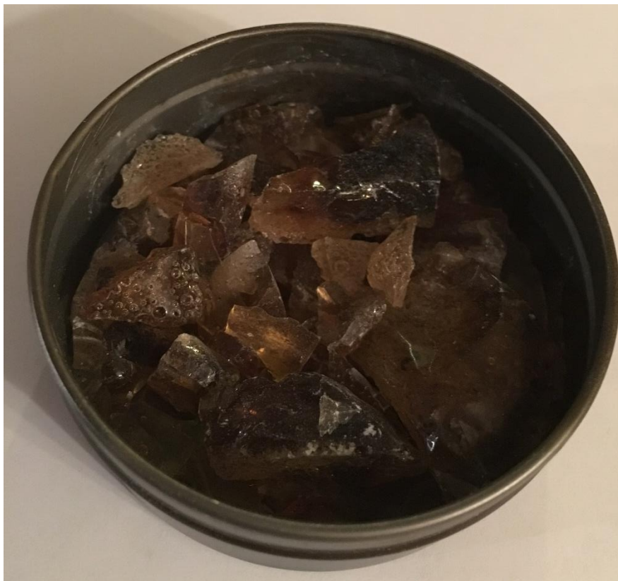
Figure 9 Densified Styrofoam after heating at 150°C.
