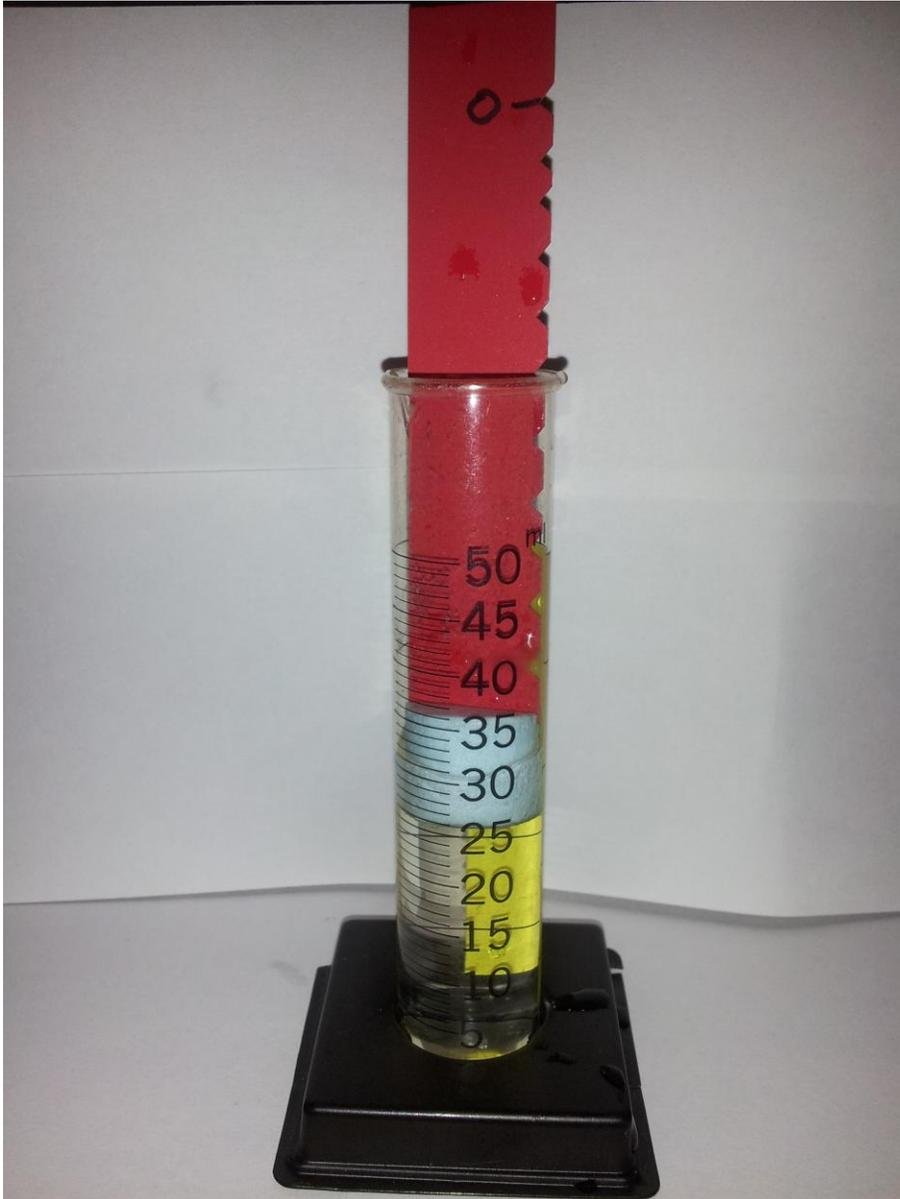
You can create a tactile adaptive graduated cylinder by cutting 5 ml. notches in a plastic strip, attaching it to a Styrofoam disk, and placing it in the cylinder. It floats when liquid is added! (Developed at Lawrence Hall of Science)
