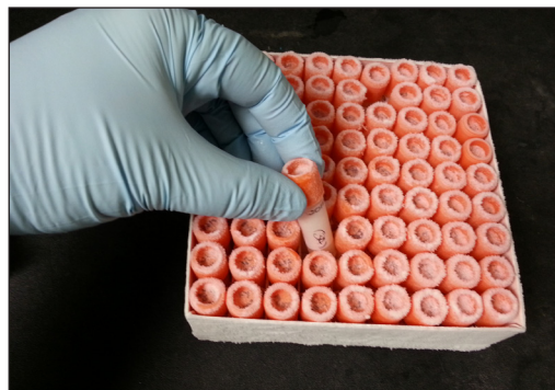
Figure 7. Cryogenic vials containing stocks of a virus can be preserved indefinitely by flash freezing and storage in liquid nitrogen. Credit: Margaret Shirra.
