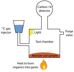
Figure 3. Set-up of PR experiment.
