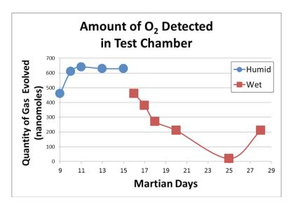
Figure 6. Levels of O<sub>2</sub> obtained during the GEx experiment. Figure adapted from Tables 4 and 5 of H.P. Klein et al. (1976), The Viking biological investigation: Preliminary results, *Science* 194(4260): 99–105. DOI: 10.1126/science.194.4260.99.
