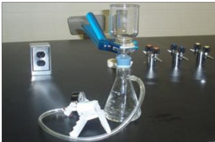
Figure 6. Apparatus for membrane filtration method
