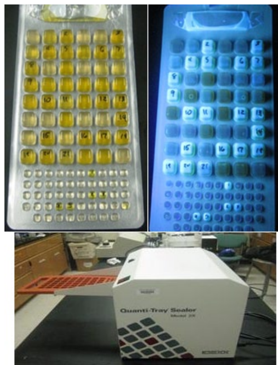
Figure 8. Quanti-Tray sealer and two Quanti-Trays that are positive for total coliform (yellow) and E. coli (glowing).
