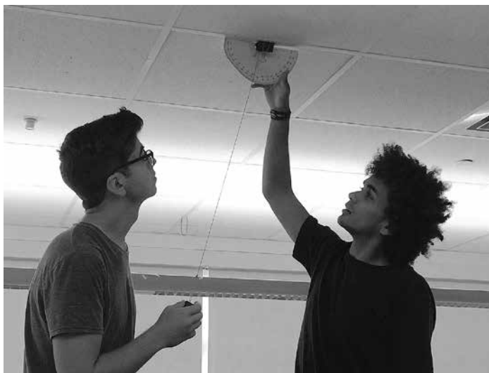
Students ready to collect data again after modifying the length of the pendulum from previous trials
