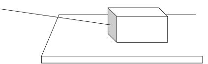
The string can be pulled slowly and the block will move. What will happen if the string is pulled very quickly? The block will resist accelerating and the string will break, following Newton's first law, part one.
