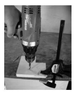
Using a clamp or clamps is one alternative to holding parts by hand. Several types of clamps are available and can be found in most hardware stores. The wood is shown clamped down to a workstation. This is more secure and safe than holding it in your hand and will yield greater precision in cuts and drilled holes.
