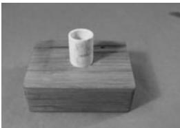
4. If the block is more than ½ inch thicker than the coupler, use a small handsaw to cut the PVC connector in half so that you have 2 rings. You will set 1 piece of the connector into each side of the block. If the block is large enough, 2 whole couplers can be used.
