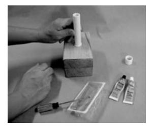
9. After the glue has dried, the block should slide on the tube with some effort. If it is too hard to move the block, it can be made easier by sanding the inside of the PVC coupler. Do not make it too easy, or the demonstration will not work. Varnish the block to seal the wood and give it a nicer appearance.
