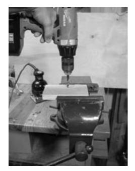
Using a vise is the safest and most secure method for holding pieces of wood during construction.
