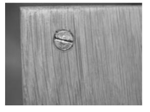
The face of the screw should be slightly beneath the surface of the wood into which it is screwed. This will keep the sharp edge of the screw head from scratching against other surfaces.
