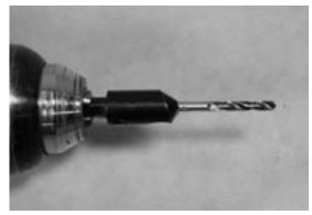
Screws put into an ordinary hole can split the wood due to the large screw-head size. The countersink drill bit will drill a hole for the shaft of the screw. The black portion of the countersink should be drilled into the wood deep enough to fit the head of the screw.
