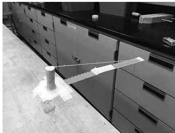
Students using pennies to anchor the cantilever
