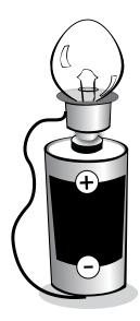
touching the bottom of the battery, touch the tip of the base of the lightbulb to the positive terminal (bumpy end) and the bulb will light.
