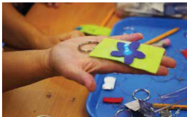
Students use conductive thread, LEDs, and coin batteries to stitch their own light-up key chains.
