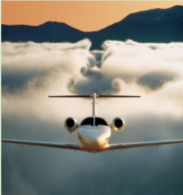
Here's the simple reason airplanes can fly: Airplane wings push down on air, which pushes back. This plane just skimmed over some fog. Its downwash (downward motion of air) is recorded as a trough; the upwash is apparent in the rising, curled edges.
