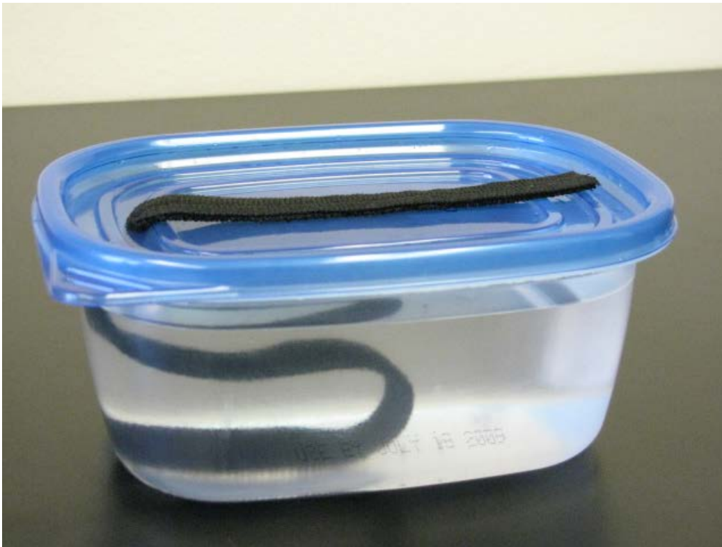
Figure 4.8. MHC Watercooler Made From a Repurposed Sandwich Meat Container and a T-Shirt Fabric Wick
