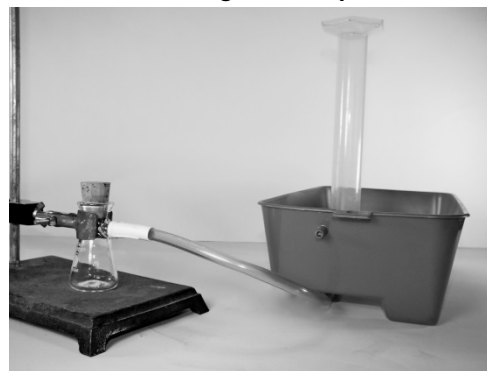
Gas collection using water displacement
