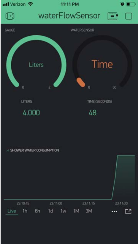
Image 1: Shows App at 4L water usage, after 2L(400 rotation) threshold has been met.
