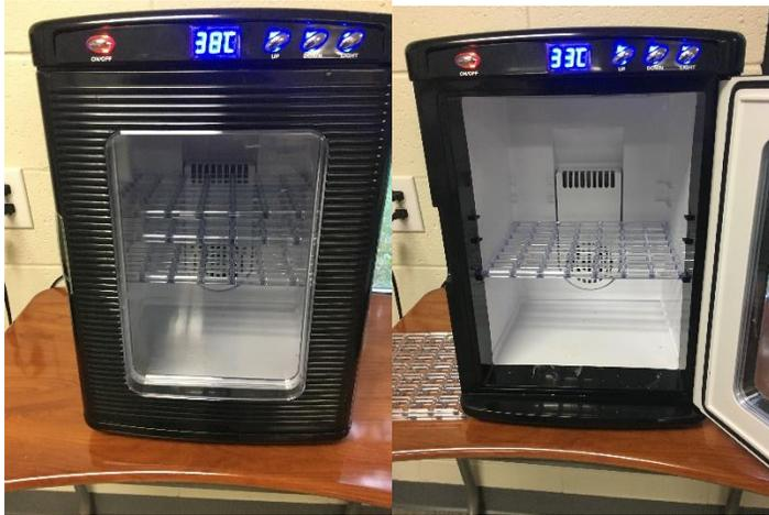
Figure: Type of low capacity table-top Incubator used in yogurt production, door closed (left), door open (right)
