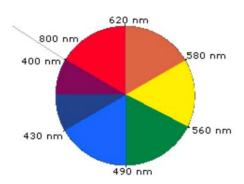
Complementary colors are diametrically opposite each other on the color wheel. Thus, absorption of 420-430 nm light renders a substance yellow, and absorption of 500-520 nm light makes it red. Green is unique in that it can be created by absorption close to 400 nm as well as absorption near 800 nm.
