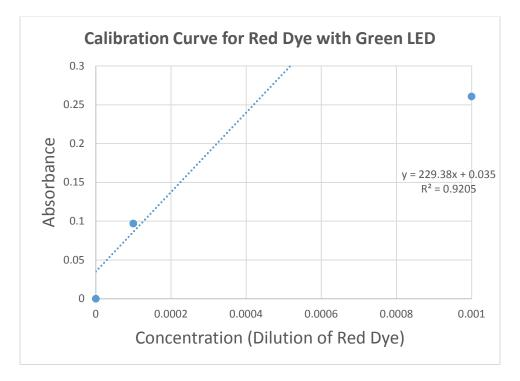
The Green LED light did not work well for any dye colors at the more concentrated solutions. In part, this might be because the green LED is much dimmer compared to the red and yellow LEDs. Not enough light seems to penetrate the more concentrated dye solutions.
