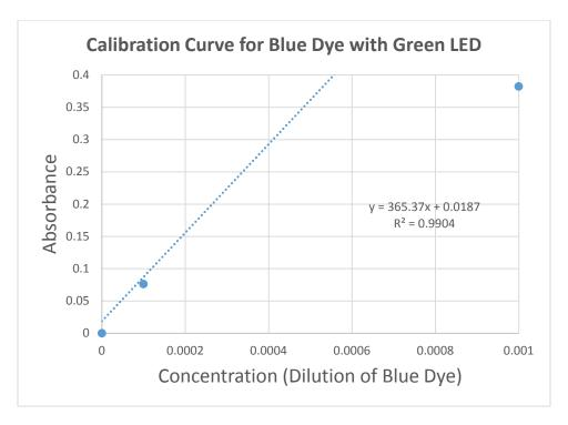
The Green LED light did not work well for any dye colors at the more concentrated solutions. In part, this might be because the green LED is much dimer compared to the red and yellow LEDs. Not enough light seems to penetrate the more concentrated dye solutions.
