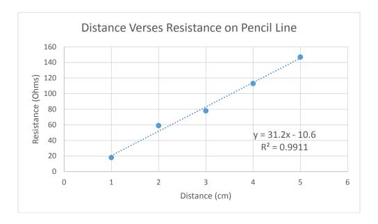
Note: the graph shows how longer distances have more resistance, which is a measure of the electrical "friction" as electrons move through a conductor.
