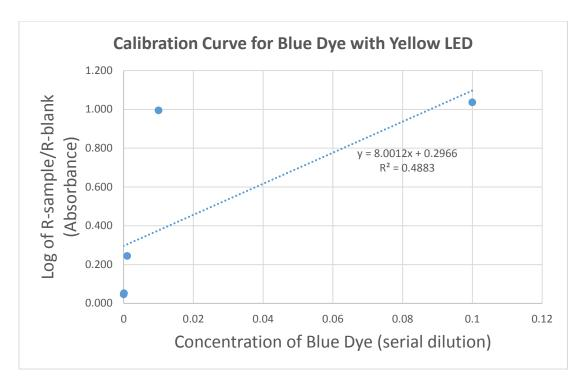
The Yellow LED light shows changes in absorbance for the blue dye but not as well as for the red dye. Note the poor R-squared value (0.488), which reflects that fewer points fall on the regression line.
