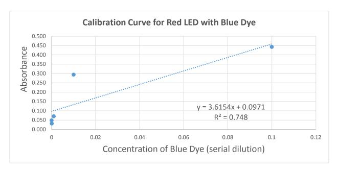
The RED LED light shows some changes in absorbance for the blue dye but not as well as for the green dye. Note the poor R-squared value (0.748). The closer this number is to 1.0 the better the fit and the more data points that fall on the regression line.
