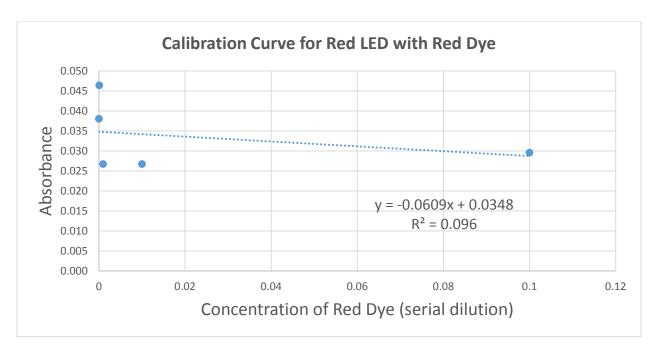
The RED LED light shows basically no change in resistance for the red dye. This is because red LED's emit light wavelengths that are reflected by the red dye (and not absorbed).
