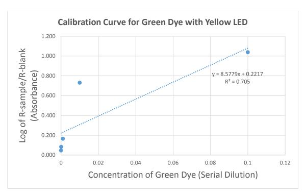
The Yellow LED light shows changes in absorbance for the green dye but the data collected does not fit the line very well, as noted by the poor R-squared value (0.705).
