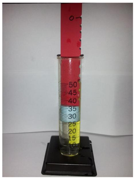
You can create a tactile adaptive graduated cylinder by cutting 5 ml. notches in a plastic strip, attaching it to a Styrofoam disk, and placing it in the cylinder. It floats when liquid is added! (Developed at Lawrence Hall of Science)
