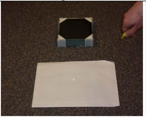
*Figure 3b Diffuse reflection: The laser pointer is directed towards the white paper screen. From there the light is reflected in all directions including the direction of the camera. So the light spot is visible from all sides.*
