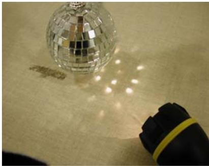
*Figure 4: Example of mirror reflection from the disco ball and diffuse reflection from the paper.*
