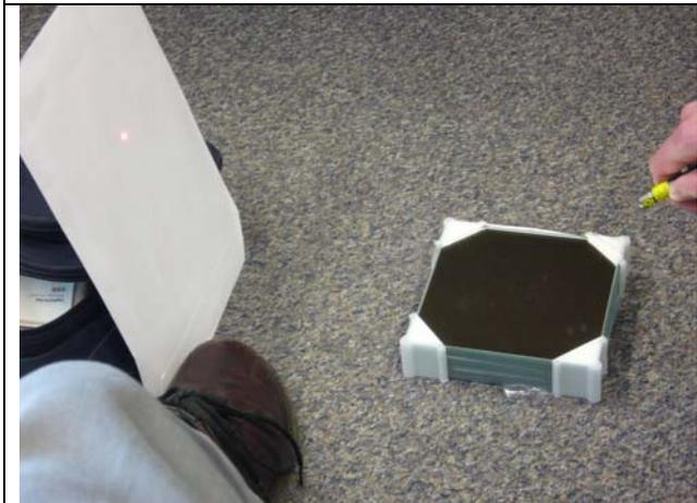
*Figure 3a Mirror reflection: The laser pointer is directed at the mirror. However, looking from the side we do not see a lighted spot on the mirror. All the laser light is reflected in one direction only, towards the white paper screen. On the screen we see a light spot as the screen reflects the light diffusely to all directions including the direction of the camera*
